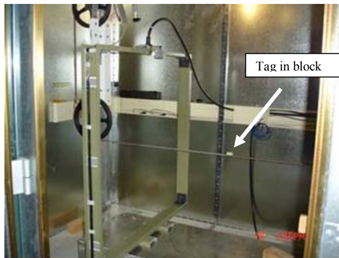
Figure 2. Photo showing the large antenna and how read-range distances were measured with tags placed along the Z-axis out from the center of an antenna.
