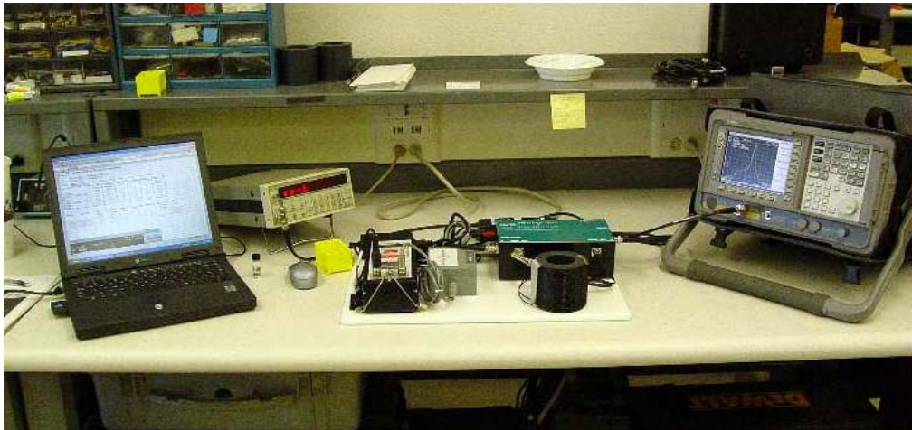
Figure 1. Photo showing the setup used by PSMFC to measure the electrical parameters.
